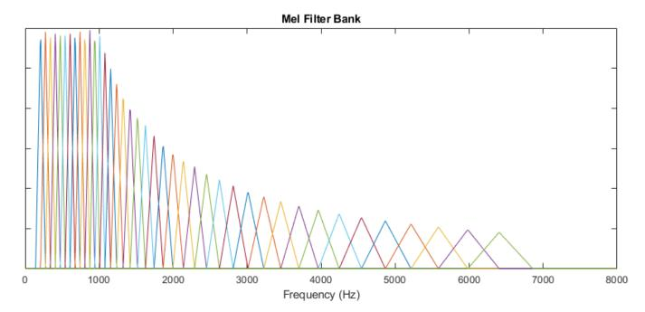
The information contained in the zeroth mel frequency cepstral coefficient is often augmented with or replaced by the log energy. The log energy calculation depends on the input domain.
