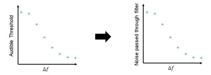
The derivative of the function relating  $\Delta f$  to the noise passed through the filter estimates the auditory filter shape. Because  $\Delta f$  has an inverse relationship with the noise power passed through the filter, the derivative of the function must be multiplied by -1. The resulting auditory filter shape is usually approximated as a roex filter.
