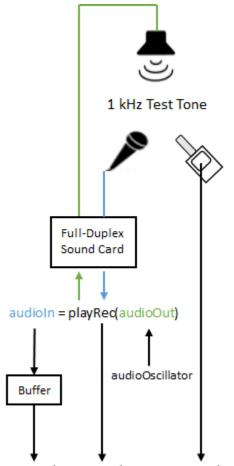
calibrationFactor = calibrateMicrophone(micRecording, sampleRate, SPLreading)
