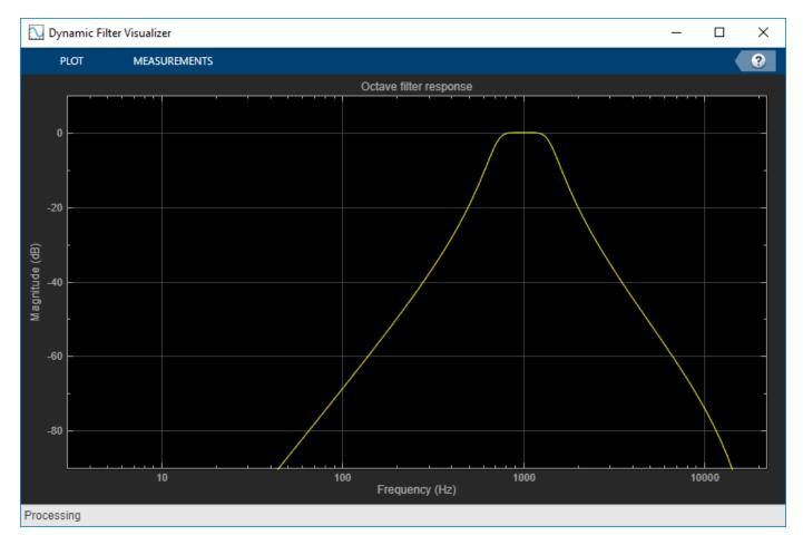
Call parameterTuner to open a UI to tune parameters of the octaveFilter while streaming. parameterTuner(octFilt)
