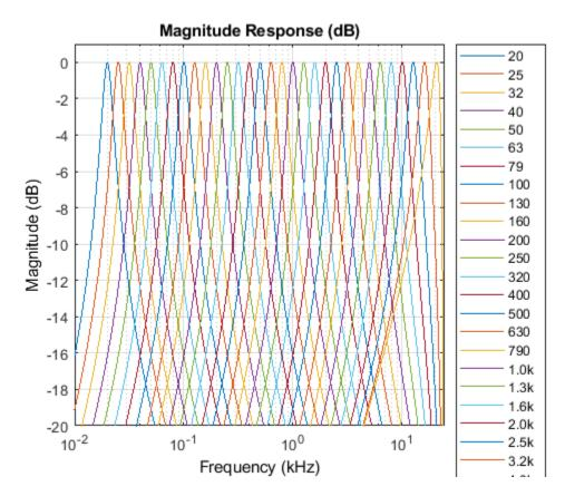
Process white Gaussian noise through the filter bank. Use a spectrum analyzer to view the spectrum of the filter outputs.
