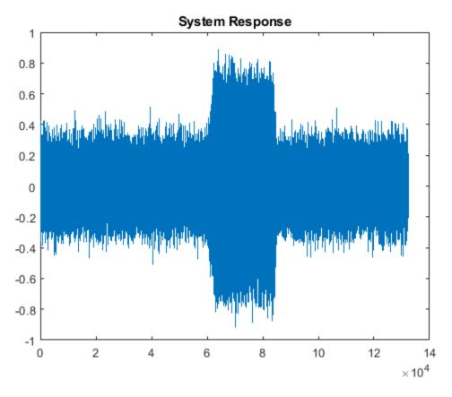
Pass the excitation signal and the system response to the impzest function to estimate the impulse response. Truncate the estimate to 100 points. Use impz to determine the true impulse response of the system. Plot the true impulse response and the estimated impulse response for comparison.
