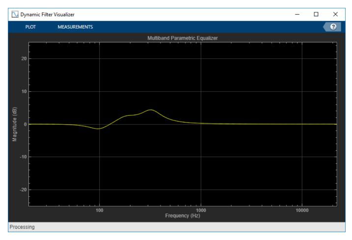
Call parameterTuner to open a UI to tune parameters of the equalizer while streaming. parameterTuner(equalizer)
