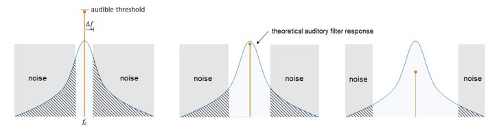
The notched-noise method assumes the audible threshold corresponds to a constant signal-to-masker ratio at the output of the theoretical auditory filter. That is, the ratio of the power of the  $f_{\rm c}$  tone and the shaded area is constant. Therefore, the relationship between the audible threshold and  $2\Delta f$  (the notch bandwidth) is linearly related to the relationship between the noise passed through the filter and  $2\Delta f$ .
