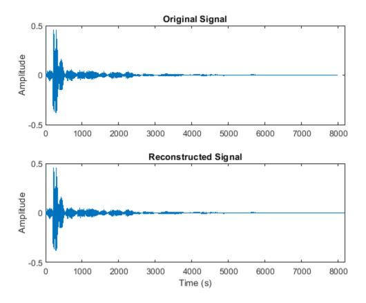
The reconstructed signal is padded with zeros at the back end. Remove the zero-padding from the reconstructed signal, plot the original and reconstructed signal, and then display the reconstruction error.
