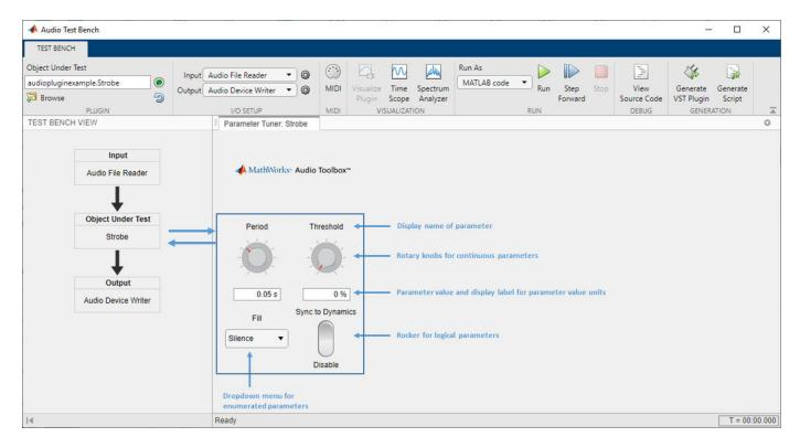
**MATLAB Environment Using parameterTuner.** Use parameterTuner to interact with plugin parameters in the MATLAB environment while developing, analyzing, or using your plugin in a programmatic workflow. The parameterTuner honors the graphical user interface you specified in audioPluginParameter, audioPluginGridLayout, and audioPluginInterface (except for filmstrips).
