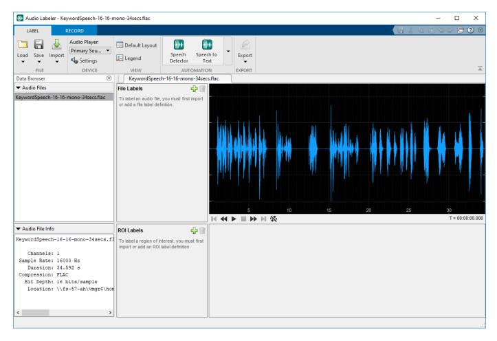
Under **Automation**, click **Speech to Text**. On the **Speech to Text** tab, select your preferred speech-to-text API. This example uses the IBM speech-to-text API. Select **Segment Words** so that the text labels are divided into individual words instead of sentences. Click **Run** to interface with the speech-to-text API and create a new region of interest (ROI) label. The ROI label contains words detected and labeled by IBM's speech-to-text API.
