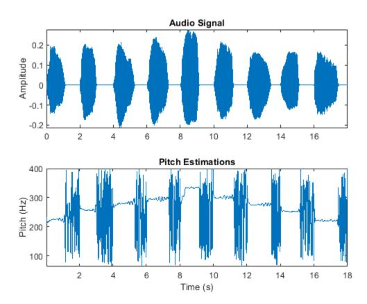
The pitch function estimates the pitch for overlapped analysis windows. The pitch estimates are only valid if the analysis window has a harmonic component. Call the harmonicRatio function using the same window and overlap length used for pitch detection. Plot the audio, pitch, and harmonic ratio.
