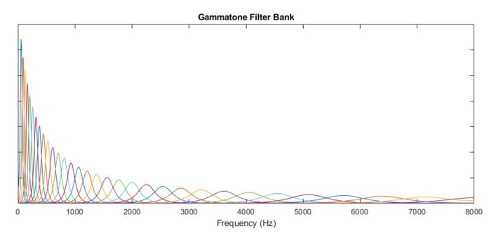
The information contained in the zeroth gammatone cepstral coefficient is often augmented with or replaced by the log energy. The log energy calculation depends on the input domain.
