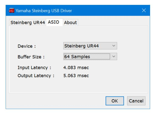
The latency is now minimized for the frame size of 64 samples. If you want to measure the reduction in latency specific to your system, follow the steps in the "Measure Audio Latency" example.
