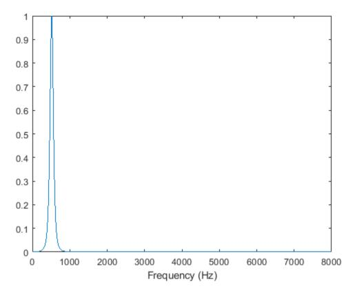
To specify the number of FFT points used to compute the frequency response, use the NFFT name-value pair. Specify that the frequency response is calculated using a 128-point FFT. Plot the magnitude frequency response.
