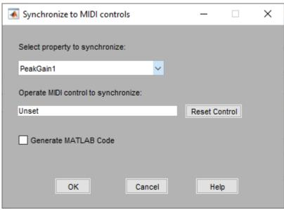
On your MIDI device, operate the control that you want to synchronize to the selected plugin property. The control appears in the **Operate MIDI control to synchronize** box.
