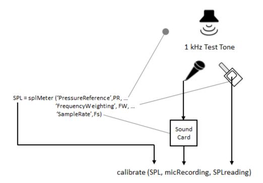
The CalibrationFactor property is set according to the equation:
