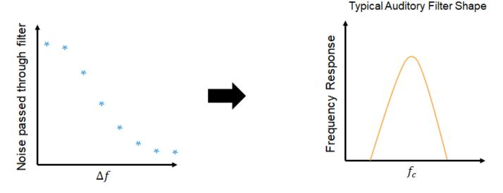
The equivalent rectangular bandwidth of the auditory filter is defined as the width of a rectangular filter required to pass the same noise power as the auditory filter.
