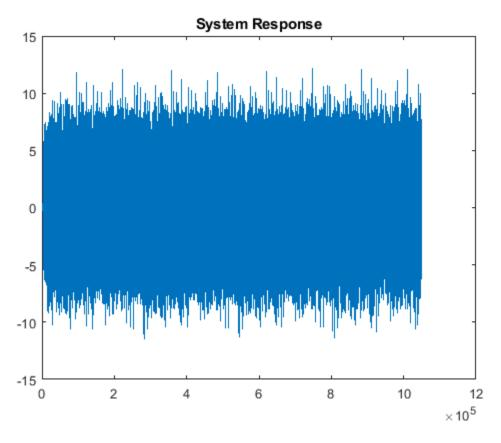
In a real-world scenario, the MLS sequence is played back in the system under test while recording. The recording would be cut so that it begins at the moment the MLS sequence is picked-up and truncated to last the duration of the repeated sequence.
