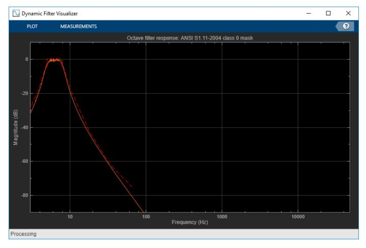
The red mask on the plot defines the bounds for the magnitude response of the filter. The magnitude response of this filter goes below the lower bound of the compliance mask between 5.5 and 7.5 Hz.
