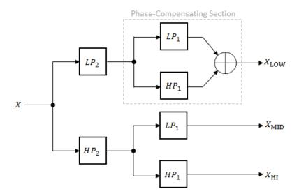
The phase-compensating section is equivalent to an allpass filter.
