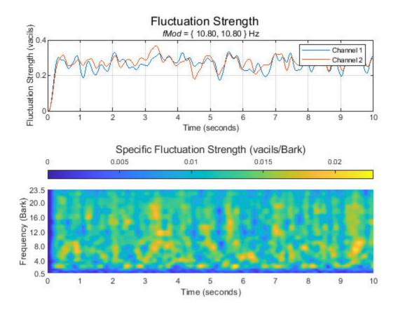
Specify the known modulation frequency and then plot the acoustic fluctuation again.
