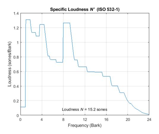
acousticLoudness enables you to specify an intermediate representation, sound pressure levels, instead of a time-domain input. This enables you to reuse intermediate SPL calculations. Another advantage is that if your physical SPL meter does not report loudness in accordance to ISO 532-1 or ISO 531-2, you can use the reported 1/3-octave SPLs to calculate standard-compliant loudness.
