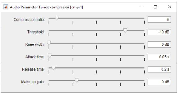
cmpr2 = compressor('SampleRate',fileReader.SampleRate);
