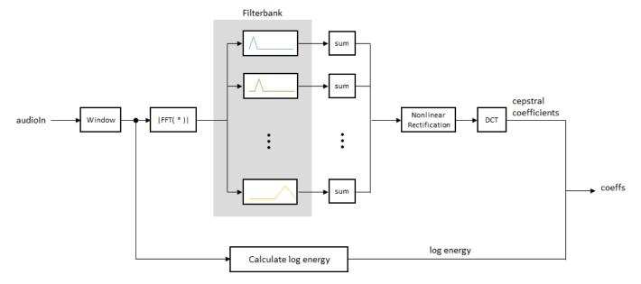
The default mel filter bank linearly spaces the first 10 triangular filters and logarithmically spaces the remaining filters.
