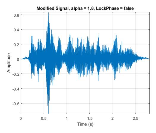
Apply the same 1.8 speedup factor to the input audio signal, this time enabling phase-locking. Listen to the audio signal and plot it over time.
