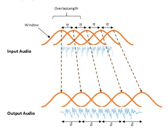
The OLA algorithm does a good job of recreating the magnitude spectra but can introduce phase jumps between windows. The WSOLA algorithm attempts to smooth the phase jumps by searching WSOLADelta samples around the  $\eta$  interval for a window that minimizes phase jumps. The algorithm searches for the best window iteratively, so that each successive window is chosen relative to the previously selected window.
