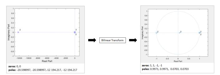
ANSI S1.42.2001 defines the weighting curve by specifying analog poles and zeros. Audio Toolbox converts the specified poles and zeros to the digital domain using a bilinear transform:
