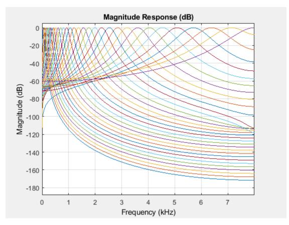
To visualize a subset of filters in the filter bank, specify the second argument as a row vector of indices between one and the number of filters in the filter bank. If not specified, fvtool visualizes 1 to N filters of the filter bank, where N is the smallest of gammaFiltBank.NumFilters and 64. Visualize the ninth filter.
