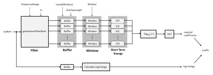
The FrequencyRange and sample rate (fs) parameters are set on the filter bank using the name-value pairs input to the gtcc function. The number of filters in the gammatone filter bank is defined as hz2erb(FrequencyRange(2)) - hz2erb(FrequencyRange(1)). This roughly corresponds to placing a gammatone filter every 0.9 mm in the cochlea.
