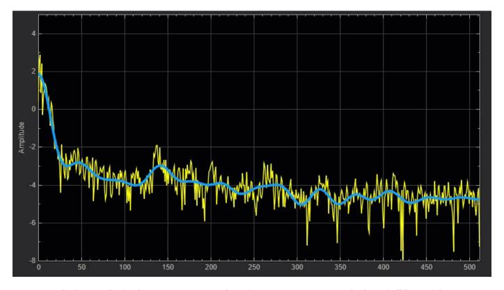
The loop ends if either a maximum number of iterations (100) is reached, or if all bins of the estimated log envelope are within a given tolerance of the original log spectrum. The tolerance is set to  $log(10^{(1/20)})$ .
