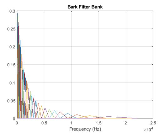
To apply frequency domain filtering, perform a matrix multiplication of the filter bank and the left and right power spectrograms.
