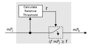
**a** The relative threshold,  $\Gamma$ , is computed:
