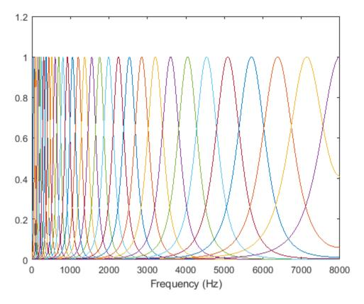
To get the frequency response of a subset of filters in the filter bank, specify the second argument as a row vector of indices between one and the number of filters in the filter bank. Get the frequency response of the 10th filter in the filter bank and plot the magnitude frequency response.
