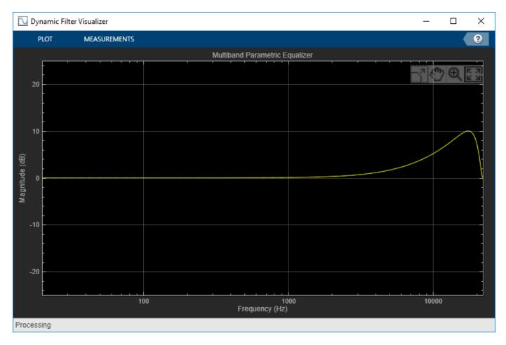
The equalizer band is warped.
