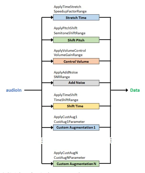
In this pipeline configuration, these parameters apply:
