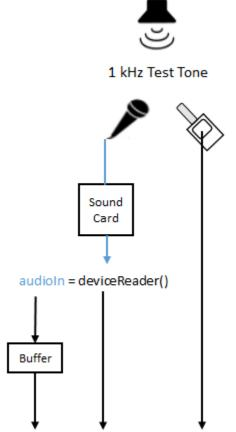
calibrationFactor = calibrateMicrophone(micRecording, sampleRate, SPLreading)
