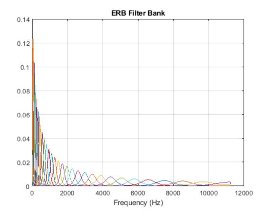
To apply frequency-domain filtering, perform a matrix multiplication of the filter bank and the power spectrogram.
