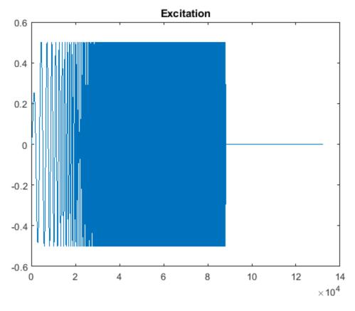
Pass the excitation signal through an infinite impulse response (IIR) filter and add noise to model a real-world recording (system response).
