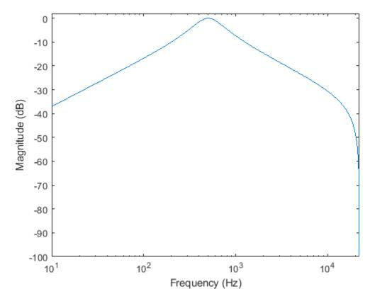
To specify the number of FFT points used to compute the frequency response, use the NFFT name-value pair. Specify that the frequency response is calculated using a 8192-point FFT. Plot the magnitude frequency response in dB.
