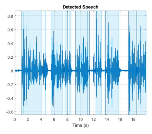
The detectSpeech function uses a thresholding algorithm based on energy and spectral spread per analysis frame. You can modify the Window, OverlapLength, and MergeDistance to fine-tune the algorithm for your specific needs.
