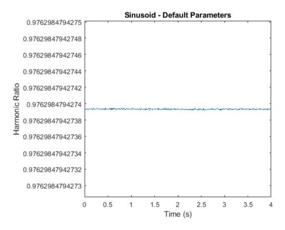
The short-time analysis required for windowing lowers the harmonic ratio from the theoretical value of 1. To diminish the effect of windowing, you can increase the window size. Use a 100 ms Hamming
