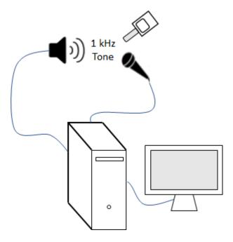
Create an audioDeviceReader object to read from the microphone and an audioDeviceWriter object to write to your speaker.
