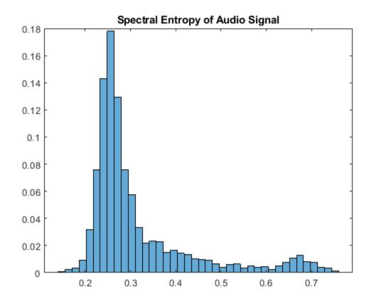
Depending on your application, you might want to extract spectral entropy from only the regions of speech. The resulting statistics are more characteristic of the speaker and less characteristic of the channel. Call detectSpeech on the audio signal and then create a new signal that contains only the regions of detected speech.
