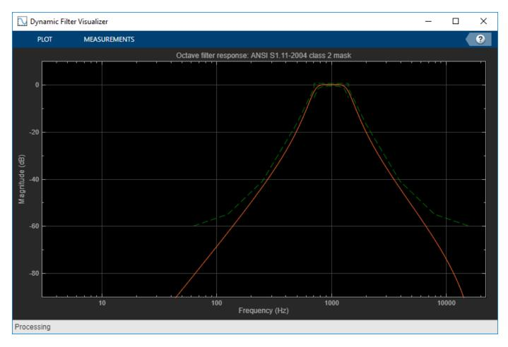
Analyze the filter using fvtool.
