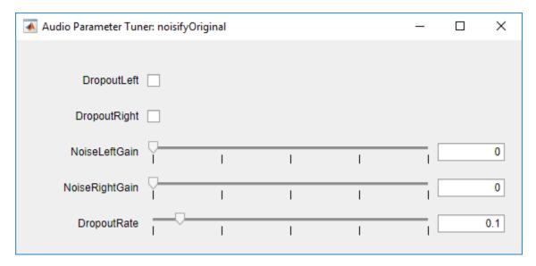
You can create a more intuitive and visually pleasing UI using audioPluginInterface, audioPluginGridLayout, and audioPluginParameter. For example, to create a more intuitive UI for noisyOriginal, you could update the audioPluginInterface as follows:
