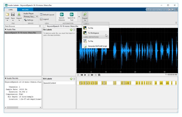
The labels are exported to the workspace as labeledSignalSet object with a time stamp. Set the variable labeledSet to the time-stamped labeledSignalSet object.
