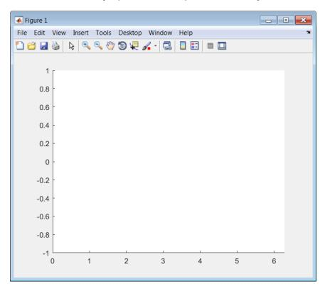
Use the midicallback function to associate your sinePlotter function with the control specified by your midicontrolsObject. Move your specified MIDI control. The plot updates automatically with the sinusoid amplitude specified by your MIDI control.
