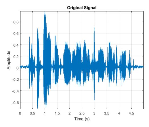
Phase-locking adds a nontrivial computational load to TSM and is not always required. By default, phase-locking is disabled. Apply a speedup factor of 1.8 to the input audio signal. Listen to the audio signal and plot it over time.
