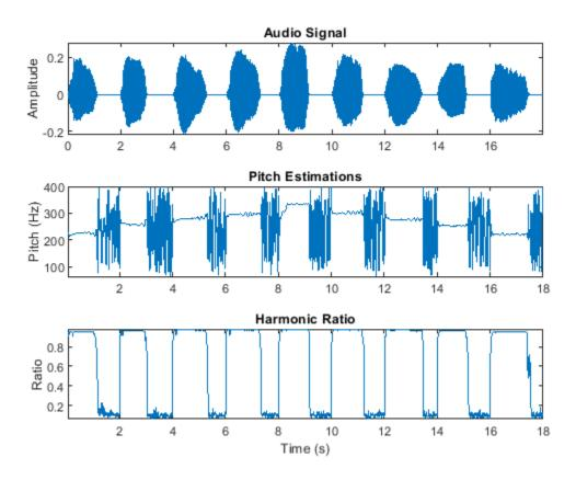
Use the harmonic ratio as the threshold for valid pitch decisions. If the harmonic ratio is less than the threshold, set the pitch decision to NaN. Plot the results.
