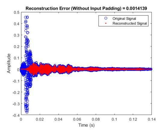
If you specify an input signal to the mdct that is not a multiple of the window length, then the input signal is padded with zeros. Pass the original unclipped signal through the transform pair and compare the original signal and the reconstructed signal.
