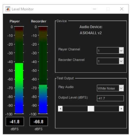
Choose a player and recorder channel, the test signal, and the output level. Verify that the level reported by the recorder reacts appropriately to level changes output by the player. Once you are
