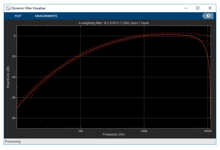
Change your A-weighting filter sample rate to  $44.1\ \mathrm{kHz}$ . Verify that the filter is standard compliant and visualize the filter design.
