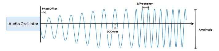
To generate tunable waveforms:
