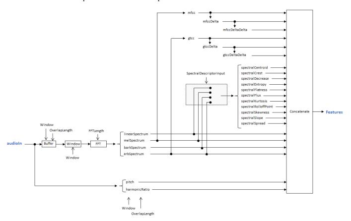
For example, to create an object that extracts the centroid of the Bark spectrum, the flux of the Bark spectrum, the pitch, the harmonic ratio, and the delta-delta of the MFCC, specify the audioFeatureExtractor as:
