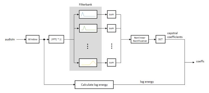
The default gammatone filter bank is composed of gammatone filters spaced linearly on the ERB scale between 50 and 8000 Hz. The filter bank is designed by designAuditoryFilterBank.
