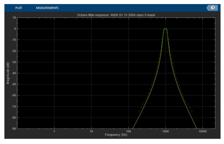
Create a spectrum analyzer to visualize the original audio signal and the audio signal after octaveband filtering.
