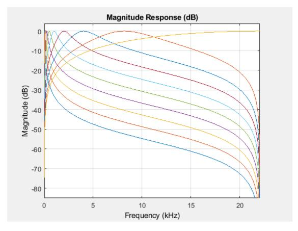
To visualize a subset of filters in the filter bank, specify the second argument as a row vector of indices between one and the number of filters in the filter bank. If not specified, fvtool visualizes 1 to N filters of the filter bank, where N is the smallest of octFiltBank.NumFilters and 64. Visualize the ninth filter.
